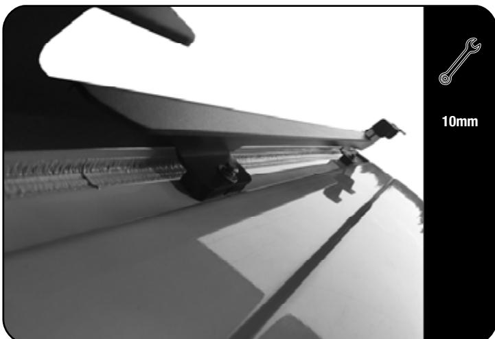
Secure the Rear Foot Rails to the vehicle with four M6 x 35 Hex Bolts, four M6 SS Spring Washers and four M6 x 19 x 1SS Flat Washers (Items 8, 9 & 10).
