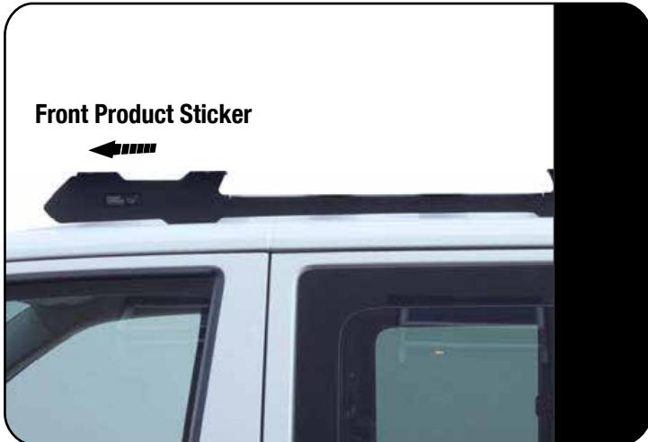
Place the Foot Rails onto the vehicle's roof, lining up the mounting holes in the bottom of the Foot Rails with the mounting points on the vehicle. The product stickers must face outwards from the vehicle as shown.
