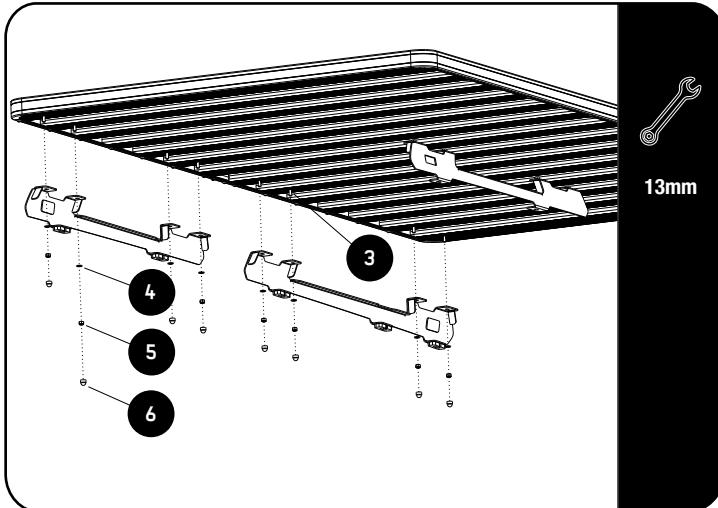
Fit your roof rack to the Foot Rails using M8 x 20 Hex Bolts, M8 x 16 x 1.6SS Flat Washers and M8 Nyloc Nuts (Items 3, 4 & 5).
