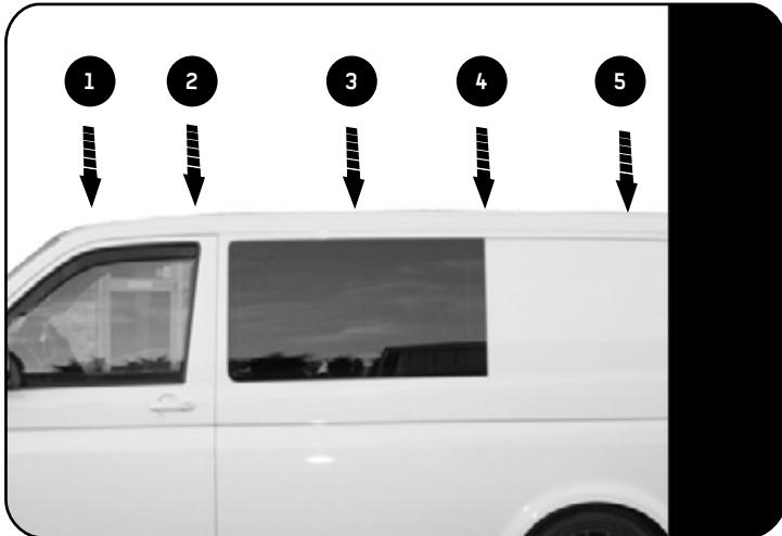
If you are installing a Full Rack remove all the OEM Plastic Button Head Bolts, but if you are installing a Half Rack remove the rear Bolts (3, 4 & 5) on the left and right hand side of the vehicle.
