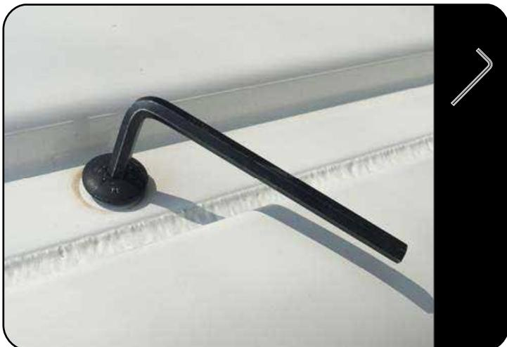
Use a 4mm Hex Allen Key to remove the above identified Bolts from the roof channel.
