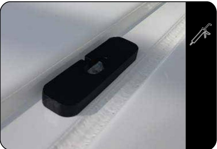
Clean the area around each of the threaded mounting pints and apply a bead of silicone on and around each point. Place a Spacer (Item 11) over each of the mounting points.
