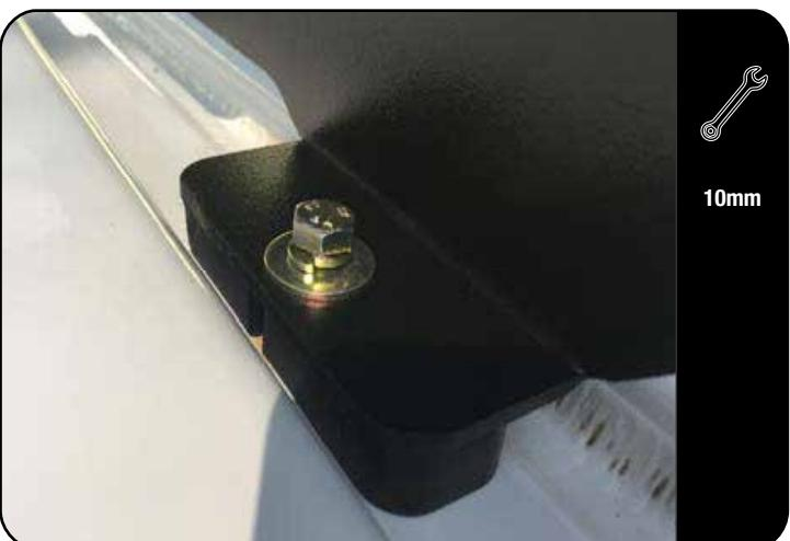
Secure the Front Foot Rails to the vehicle with four M6 x 35 Hex Bolts, four M6 SS Spring Washers and four M6 x 19 x 1SS Flat Washers (Items 8, 9 & 10).
