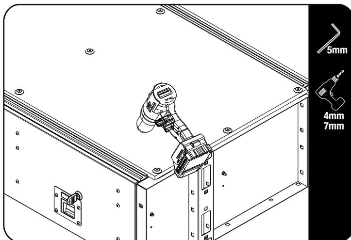
Remove the Fridge Slide and Drill a 7mm hole through the wood on each of your markings. Loosen and remove the deck. Turn the deck upside down and screw the Wood Inserts (Item 6) into each of the holes drilled in step 2.1.
