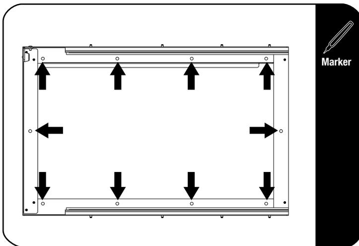
Place the Fridge Slide (Item 1) on the suitable surface, open the slide and mark the positions as shown as indicated by the arrows (at least 6 fixing points recommended).
