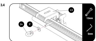
Fit and Secure the handle clamp in the desired position, using fasteners shown in Figure 1.2
