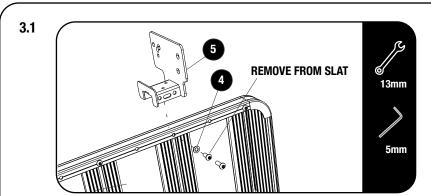
Fit and Secure Base Bracket in desired position as shown.
