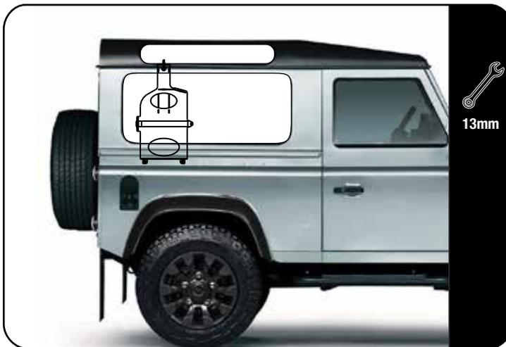
Fully tighten the gutter clamp bracket that was loosened in 2.1
