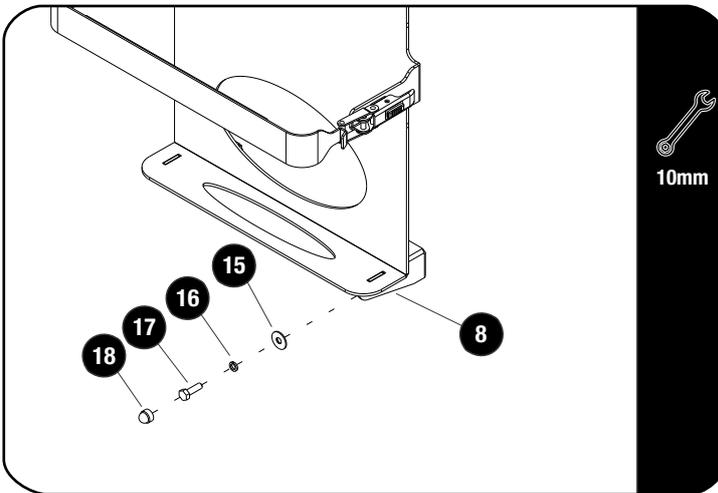
Mount the Vertical Jerry Can Holder (Item 8) to the vehicle using two M6 x 20 Hex Bolts, two M6 Spring Washers and two M6 Flat Washers (Items 15,16 & 17).
