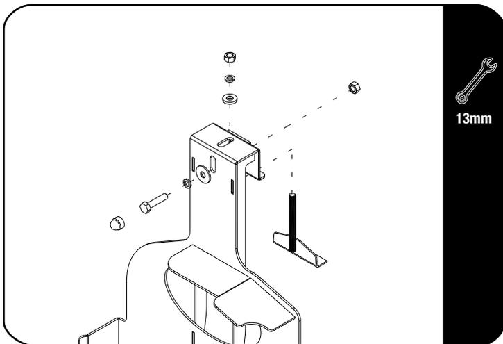
Loosen the fixings that hold the gutter clamp to the Jerry Can Holder so that it can be adjustable when placed on the vehicle.
