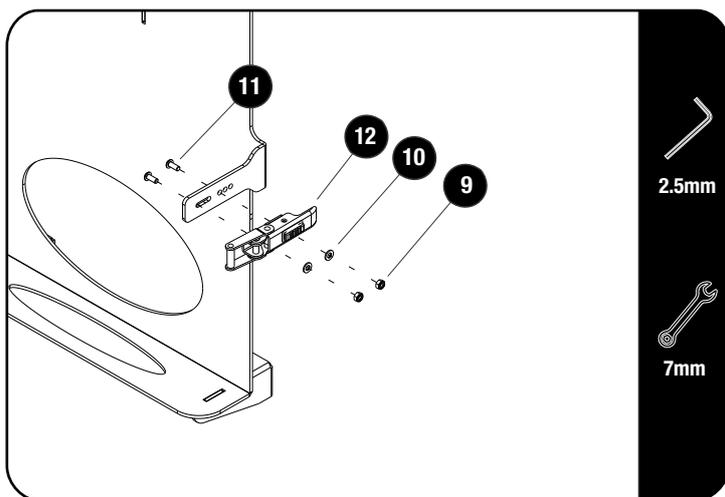
If needed adjust the Latch (Item 12) using two M4 x 10 Button head, two M4 Flat Washers and two M4 Nyloc Nuts (Items 9,11 & 11 ) so that it accommodates your Jerry Can before fully tightening.
