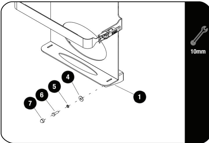
Mount the Vertical Jerry Can Holder (Item 1) to the vehicle using two M6 x 20 Hex Bolts, two M6 Spring Washers and two M6 Flat Washers (Items 6, 5 & 4).
