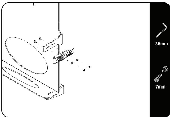
If "needed" adjust the Latch using two M4 x 10 Button head, two M4 Flat Washers and two M4 Nyloc Nuts so that it accommodates your Jerry Can.
