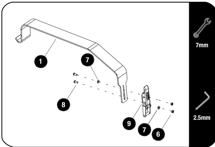
🔄 If needed, adjust the Latch (Item 9) using two M4 x 10 Button Heads, two M4 Flat Washers and two M4 Nyloc Nuts (Items 6, 7 & 8) before fully tightening.
