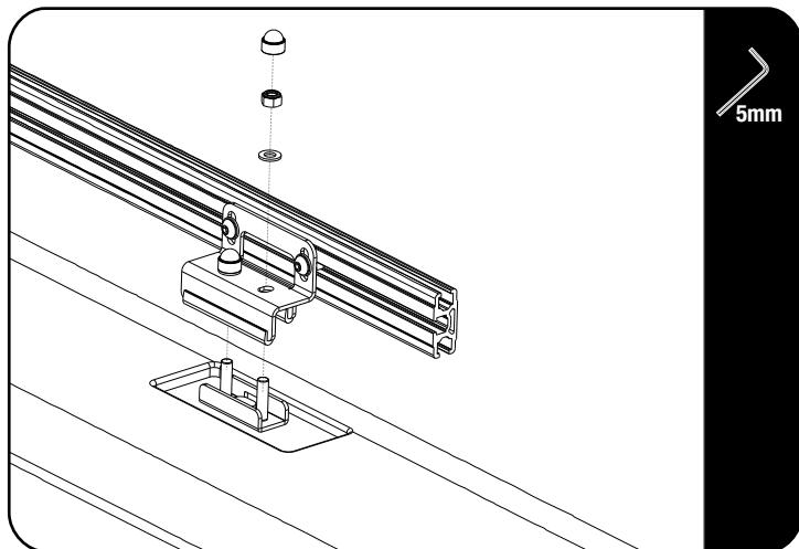
**Ensure Rubber Trim is fitted to both sides of the foot.**
