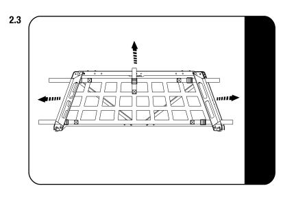
To tighten the Pro Bed Tailgate Net, pull the straps on the top and sides outward as shown.
