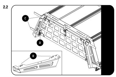
To fit the sides of the Pro Bed Tailgate Net, slide the loops on each side (C) into the corresponding slot (D) at the top and bottom of the corner brackets, as shown. Do not tighten the strap through the buckles yet.
