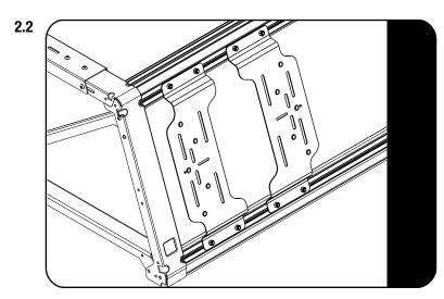
Place the Mounting Plates (Item 1) onto the M8 x 16 Hex Bolts (Item 2) and loosly fasten the Nylock Nuts (Item 4).
