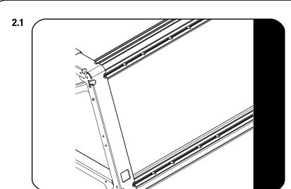
Slide four M8 x 16 Hex Bolts (Item 2) into the top side profile of your Pro Bed Rack and four M8 x 16 Hex Bolts (Item 2) into the bottom side profiles of your Pro Bed Rack as seen in Fig 2.1.
