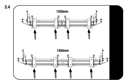
Take note of the Wolf Pack Mounting Brackets positions for 1250mm and 1450mm length extrusion.
