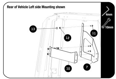
Loosely fit the Mount Bracket RH (Item 7) to the inside of the leg mount as shown using M6 x 16 Button head screw and M6 nyloc nut (Item 11 & 12).DO NOT TIGHTEN.
