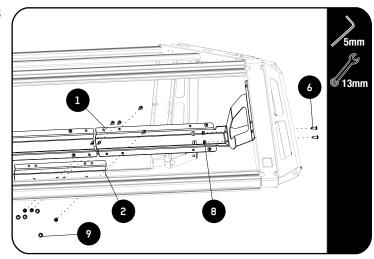
Loosely assemble the two U-Channel
