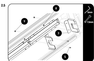
Fit the Wolf Pack Mounting Bracket (Item 3) to the U-Channel Brackets as shown using the M8 x 16 Button Head Screw and M8 Nyloc Nut (Item 5 & 8).
