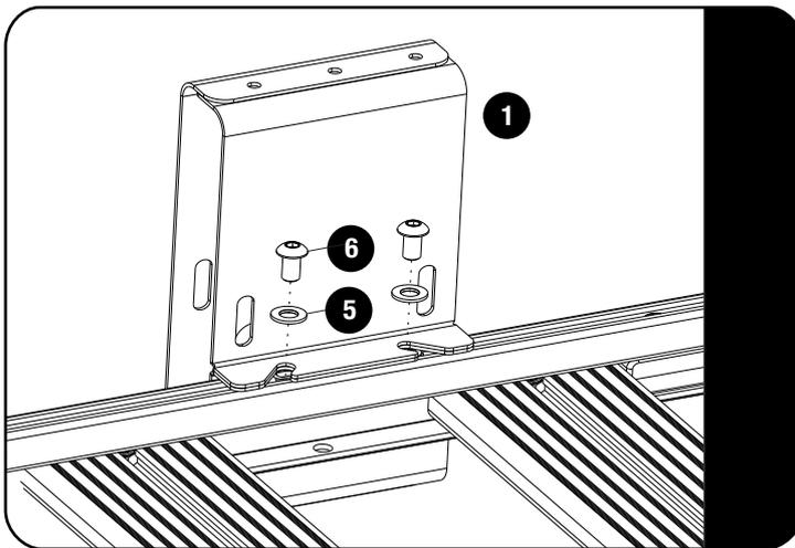
☻ Place the Head Bracket (Item 1) over the M8 Nyloc Nuts inserted in 2.1, using the M8 x 16 Button Head bolt together with the M8 Flat washer (Item 5 & 6) and hand tighten the M8 x 16 Button Head Bolt (The Bracket must be able to slide).
