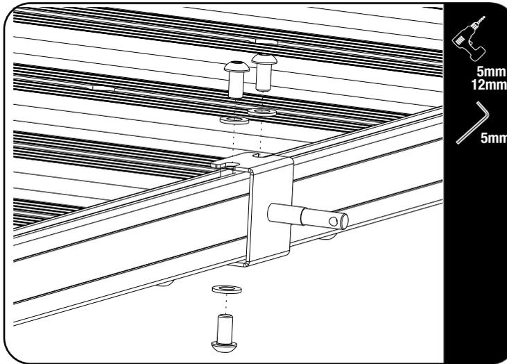
⌚ The handle bracket mounts in between 2 slats and locates in-line with the bottom hole in the side profile. Slide the handle bracket between the M8 nyloc nuts inserted in 2.1 position the axe bracket to where you would like it mounted.
