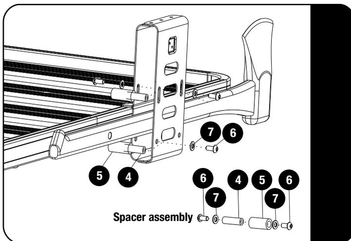
☻ Depending on which side of the Head Bracket you would like the axe handle to exit, you may need to move the 2 spacer assemblies (one to top & one bottom) to the opposite side. The spacer assemblies must be on the same side the handle exits the bracket.
