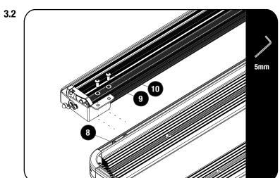
Slide four M8 Nyloc Nuts (Item 8) into the Combined Slat as shown.
