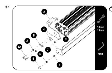
Fit the Light Cover and Cover Stopper Washer (Item 1 & 4) with the LED light to the brackets as shown, using the M6 x 16 Button Head Bolts, M6 x 12 x 1SS Flat Washers, M6 Nyloc Nuts (Item 6, 7 & 12) and fasteners supplied with the light.
