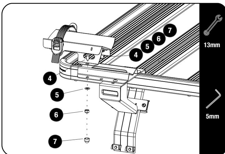
Secure the rear wheel mount bracket (included with RRAC153) to the rear assembly using M8 x 16 Button Head Bolts, M8 x 16 x 1.6SS Flat Washers and M8 Nyloc Nuts (Items 4, 5 & 6) as shown.
