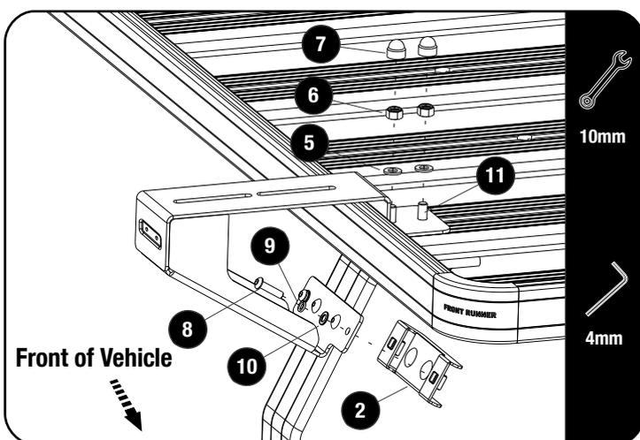
Slide two M8 x 20 Hex Bolts (Item 11) into the machined slots of the slat where the Leg is bolted to.
