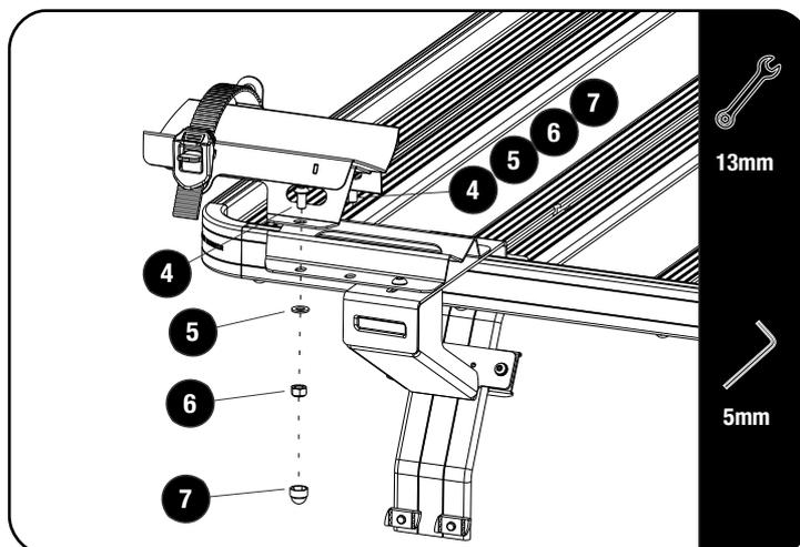
🔄 Secure the rear wheel mount bracket (included with RRAC154) to the rear assembly using M8 x 16 Button Head Bolts, M8 x 16 x 1.6SS Flat Washers and M8 Nyloc Nuts (Items 4, 5 & 6) as shown.
