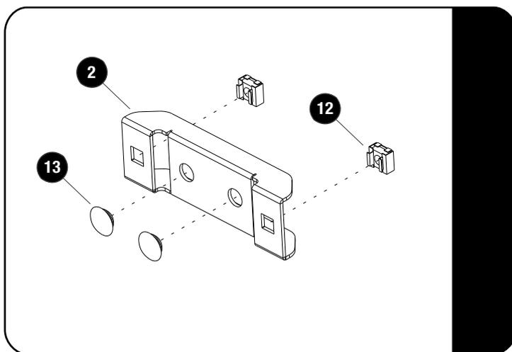
Insert two Cage Nuts and two Rubber Grommets (Items 12 & 13) into each Leg Clamp (Item 2) as shown.
