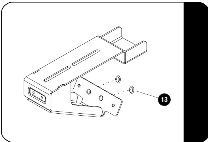
Insert two Rubber Grommets (Item 13) into each of the Side Mount Brackets (Item1).
