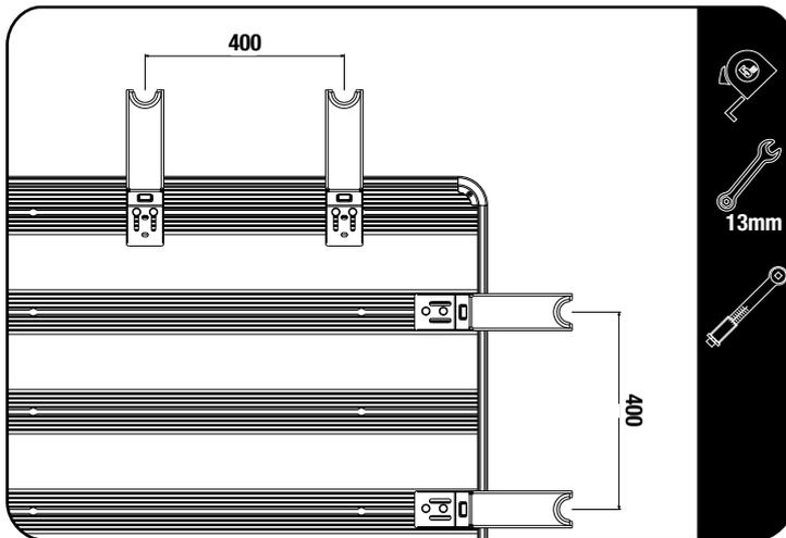
Space the Brackets 400mm apart centre to centre as shown in the illustration and tighten the M8 Nyloc Nuts. Add the M8 Nut Caps to the M8 Nyloc Nuts.
