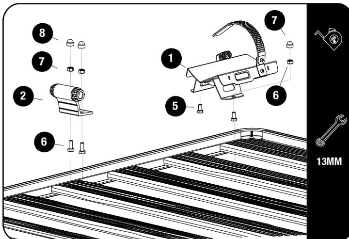
⌚ Decide where you want to mount your bike on the rack. Find the correct spacing between the fork and rear wheel. To fit the Thru Axle Bracket (Item 2), slide two M8 x 20 Hex Bolts (Item 5) into the T-slot of the chosen slat. Place the Thru Axle Bracket (Item 2) over the two Hex bolts and secure to the rack using two M8 Nyloc Nuts (Item 6) This will apply to Load Bars as well.
