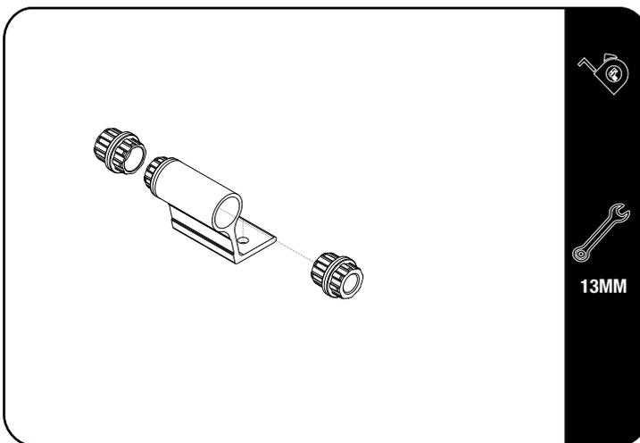
⌚ Choose which Thru Axle Insert is suitable for your bike and assemble one pair as shown.
