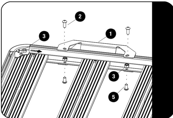
Secure the Handle Light Rack Bracket (Item 1) to your Roof Rack using M8x16 Button Heads, M8x20 Button Heads, M8x16x1.6 Flat Washers and M8 Nyloc Nuts (Items 2,3 & 5).
