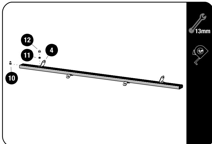
Fit the Light Bar Bracket 01 (Item 4) for for frontrunner 40" light bar, using M8x16 Hex Bolt & M8 Nyloc Nut (Items 10 & 11). Fit light bar and center on slat before fully tightening the brackets.
