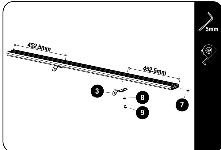
Remove the Wind Fairing Mid Support Brackets that is currently on the slat and replace it with the Fairing Mid Support Bracket supplied with this kit (Item 3).
