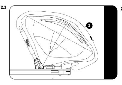
Secure the Kayak / Canoe to the Foldable Kayak Carrier Brackets (Item 1) using the Tie Down Straps (Item 2).
