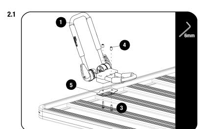
Select a suitable position on your roof rack to mount the Foldable Kayak Carrier Brackets (item 1).
