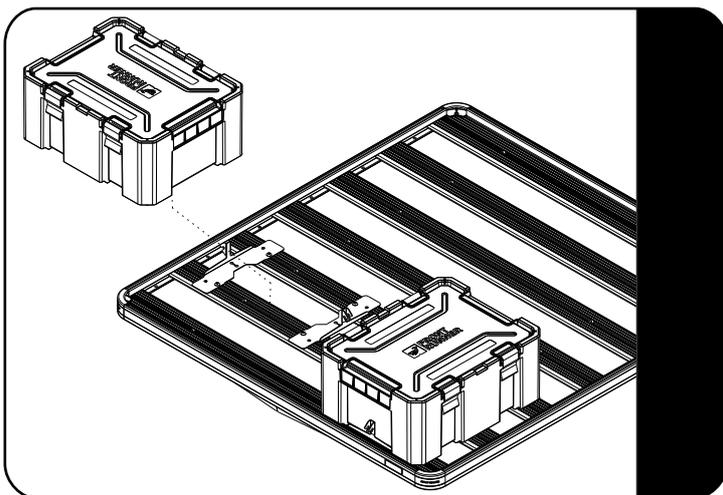
Place your Wolf Pack Pro onto the rack between the Wolf Pack Pro catch brackets. Move the brackets snugly against the Wolf Pack Pro before fully tightening.
