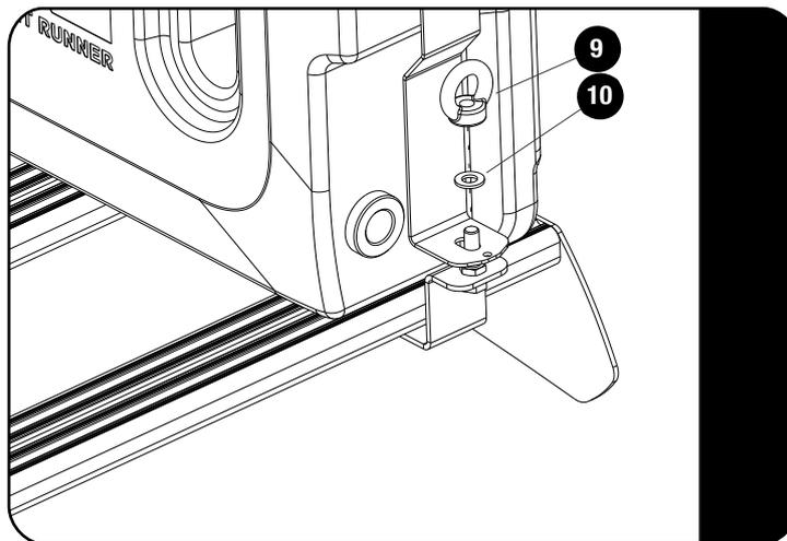
↻ Sure the front of the Strap to the M8 x 30 Hex Bolt inserted in 4.1 using a M8 Eye Nut and M8 Nylon Washer (Items 9 & 10) as shown.
