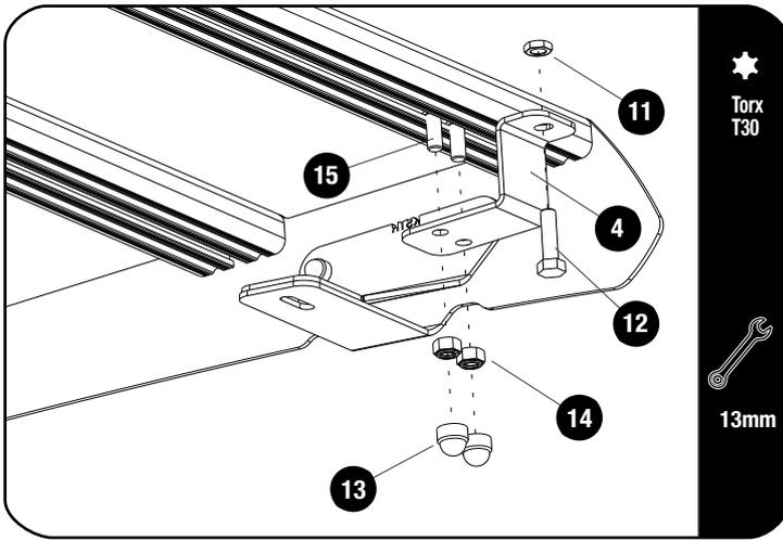
Choose where you would like to mount your Pro Water Tank Bracket. Remove the Self Forming Screws from the chosen slat, lift the slat and slide two M8x20 Hex Bolts (item 15) in the bottom T-Slot.
