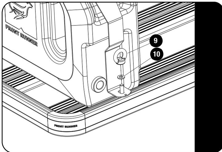
↻ Sure the front of the Strap to the M8 x 30 Hex Bolt inserted in 3.1 using a M8 Eye Nut and M8 Nylon Washer (Items 9 & 10) as shown.
