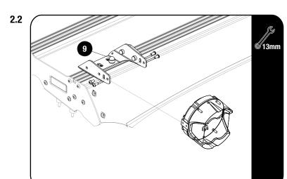
Place your LP4 Light between the Mounting and secure using the fasteners supplied with the light.
