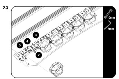
When installing multiple lights, the brackets can be linked and secured together using the supplied spacer, M6 Button Head Bolts and M6 Nyloc Nuts (Item 2,3 & 4) to form a light bar
