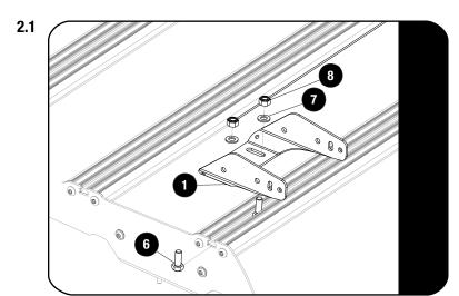
Slide M8 x 20 Hex Bolts (Item 6) into the slat as shown 2 bolts per bracket.
