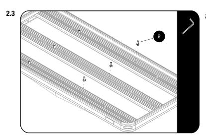
Insert two M8 x 20 Hex Bolts (Item 2) into the T-slots of three consecutive slats, in the position chosen in Step 2.1
