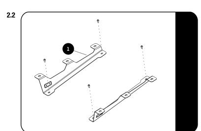
On a suitable flat surface, fit the Mounting Brackets (Item 1) to the Starlink mounting holes on the underside using the bolts (1/4 UNC x 1/2") included in your Starlink's kit.
