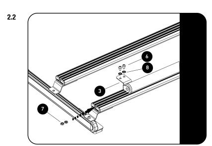
Insert four M8 Thin Nuts (Item 7), two per side into the slat's machined slots as shown.
