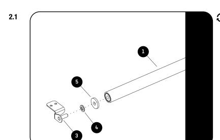
Slide the Mount Bracket together with an M12 Flat Washer and Spacer (Items 2/3, 4 & 5) into each end of the Cargo Roller (Item 1) as shown.
