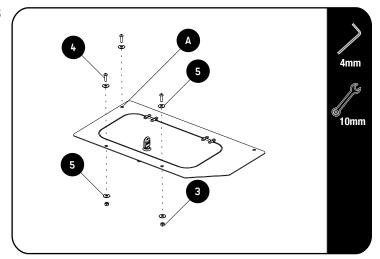
Loosely fit the Safe Assembly (Item 1) to the specified holes shown in Step 2.2.
