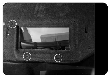
Remove the retaining clips at the specified locations marked with a circle, these holes will be the mounting points used to secure the safe to the body work of the vehicle.
