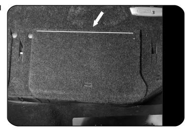
The safe must be installed below the passenger side rear seat.
