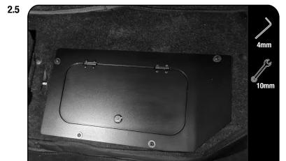
Refit the Safe Assembly (Item 1) by fully tightening all of the M6 x 20 Button Head Bolts, M6x19x1 Flat Washers & M6 Nyloc Nuts (Item 3, 4 & 5) refer to Figure 1.1 for fastener locations.
