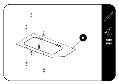
Mark mounting point (B) with a marker and remove the Safe Assembly (Item 1) so that the marked point can be drilled.
