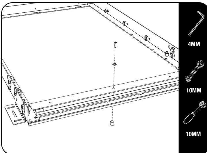
Place the frame back onto the load bed and secure using the fasteners and spacers supplied. The spacers (Item 3) are to be used when the mounting points are in a "dip" and not on a raised section by placing it over the rivnut so that the frame rests on the spacer.
