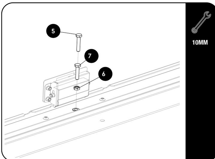
Before refitting the slide to the frame, use the M6 x 35 or M6 x 40 hex bolt (Item 5 or 7) (depending on which fits the specific vehicle best) together with the M6 Normal nut (Item 6) and assemble as shown.
