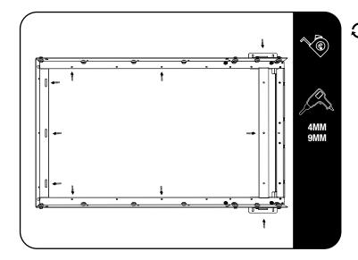
Make sure you have closed the load bed tail gate to ensure that it does not make contact with the frame. Once you are satisfied with the positioning of the frame, mark the position of all the mounting points as indicated by the arrows onto the load body.
