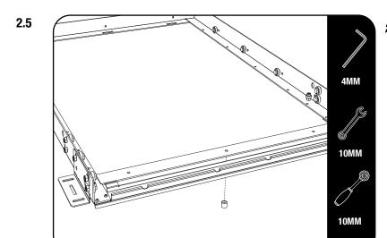
Place the frame back onto the load bed and secure using the fasteners and spacers supplied. The spacers (Item 3) are to be used when the mounting points are in a "dip" and not on a raised section by placing it over the rivnut so that the frame rests on the spacer.
