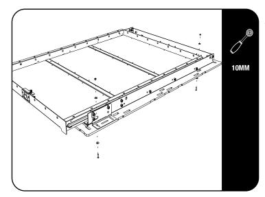
Before fitting the Cargo Slide in the vehicle, remove the wood base by loosening the four M6 Button Head Bolts.
