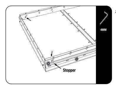
Looking at both the left and right rear corners of the Cargo Slide (Item 1), loosen and remove the rubber stopper. This is done by gripping the stopper to prevent it from t urning and removing the M6 button head bolt as shown. Once removed keep in a safe place as you will need to replace them at a later stage.
