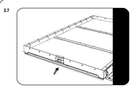
Refer to Step 2.2, refit the tray and stoppers. Once refitted check that the push to close latch engages fully and that the slide is secure.
