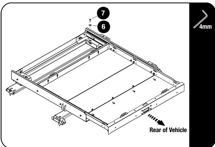
Secure the Cargo Slide using M6x16 Button Heads & M6x19x1 Flat Washers (Items 6 & 7) as shown (SSST003 sold separately).
