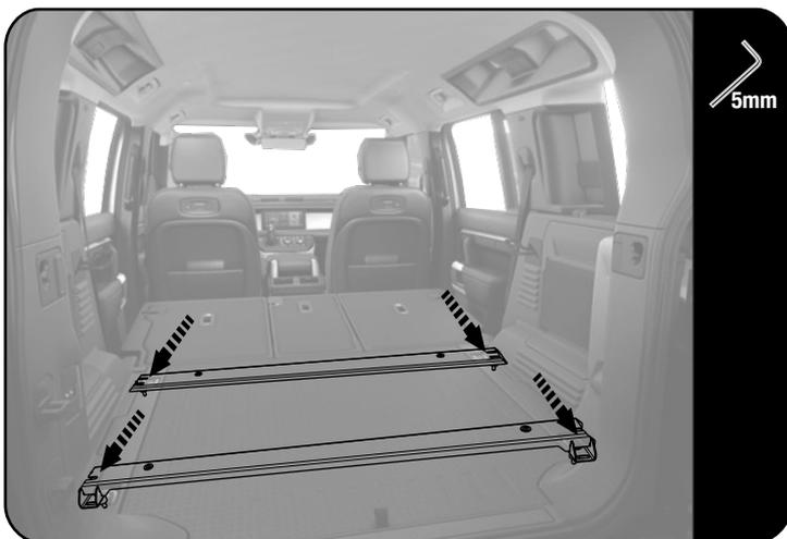
Secure both front and rear mounting plates to the existing tie down points using M8x45 Button heads, M8x19x3 Flat washers & Spacers (Items 3, 4 & 5) as shown in Fig 1.1.
