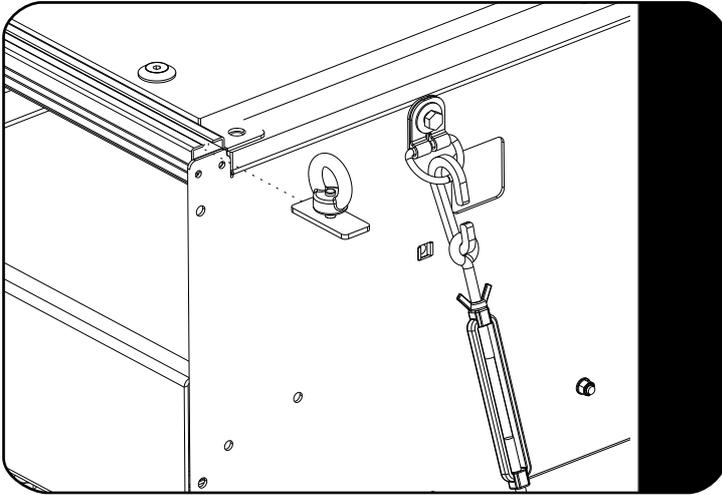
Should you wish to use the Eye Nut assemblies from step 2.2 as tie down points, they can be slid into any of the 3 top extrusions as shown and tighten in the required position.
