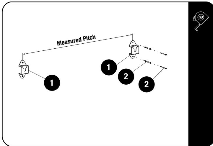
Measure the Pitch and the height in 2.4 and mark the holes of the second Wall Mount Bracket (Item 1) onto the wall.
