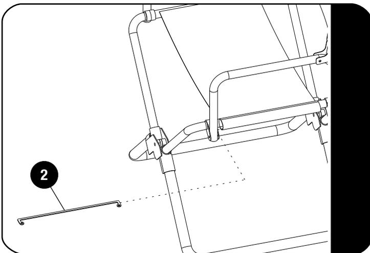
↻ Slide the Table Hinge (Item 2) in between the tube and the chair material as shown.
