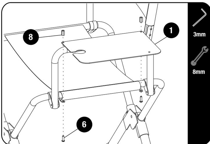
↻ Assemble the Table Top (Item 1) to the Table Hinge (Item 2) using M5 x 15 Button Head screws and Long Hex Nuts (Item 8)
