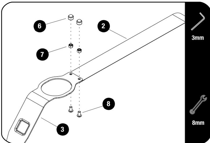
Assemble the Front and Rear Straps using M5 x 10 Button Head Bolts and M5 Nyloc Nuts (Items 7 & 8) as shown.
