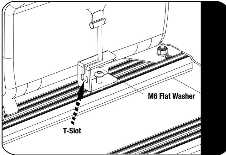
↻ Insert the Strap Assembly into the T-slot of the Rear Mount Bracket as shown.
