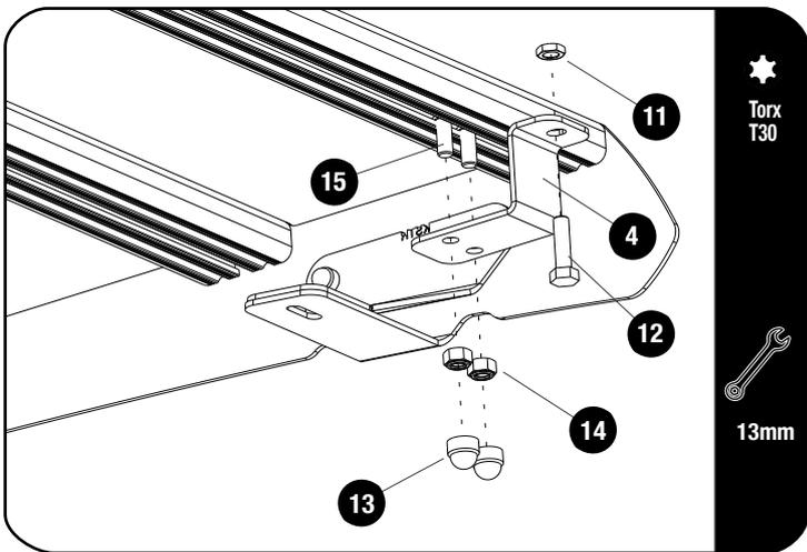
Choose where you would like to mount your Pro Water Tank Bracket. Remove the Self Forming Screws from the chosen slat, lift the slat and slide two M8x20 Hex Bolts (item 15) in the bottom T-Slot.
