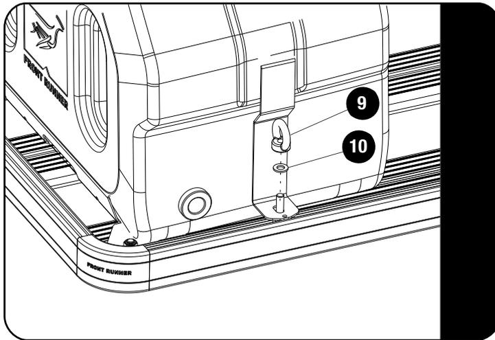
Secure the front of the Strap to the M8 x 30 Hex Bolt inserted in 3.1 using a M8 Eye Nut and M8 Nylon Washer (Items 9 & 10) as shown.
