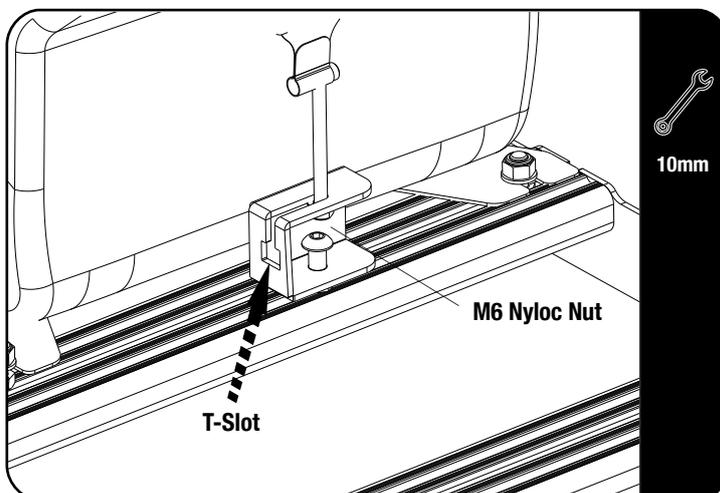
↻ Adjust the tension on the Strap by tightening the M6 Nyloc Nut. Fully Tighten the M8 Nyloc Nuts that was fitted in 4.2 to secure the Mounting cradle against the water tank.
