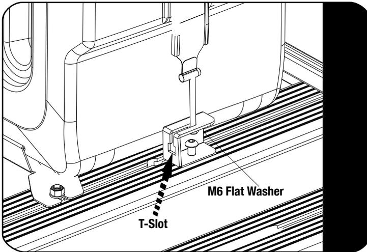
Insert the Strap Assembly into the T-slot of the Rear Mount Bracket as shown.
