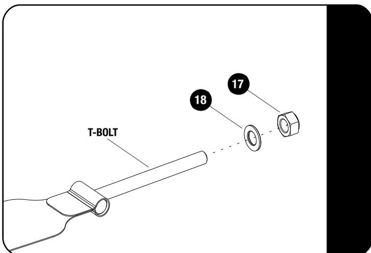
Loosely fit the M6 Nyloc Nut and M6 x 12 x 1 Flat Washer (Items 17 & 18) to the T-Bolts at the end of the Rear Strap as shown.
