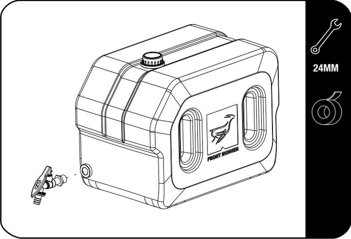
When fitting the tap, apply thread tape to the thread of the tap.
