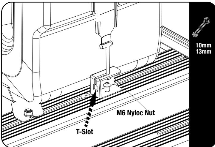
Adjust the tension on the Strap by tightening the M6 Nyloc Nut.
