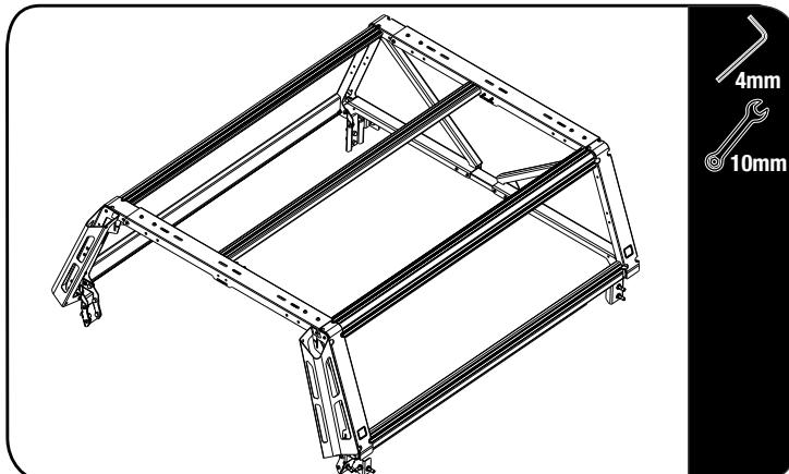
Fully tighten all the bolts and nuts and place nut caps where needed.
