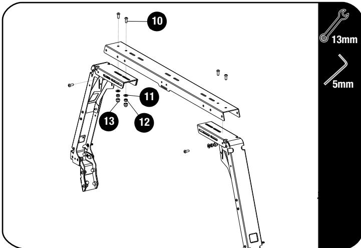
Loosely assemble the Rear Top Truss using the M8x20 Button head screws, M8x19x2 Flat washer and M8 Nyloc Nuts (Item 10,11&12).
