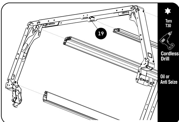
Assemble the rear Pro Bed Legs assembly to the extrusions assembled in 2.8 using the M6x25 Thread Forming screws, T30 Torx bit and a cordless driver.
